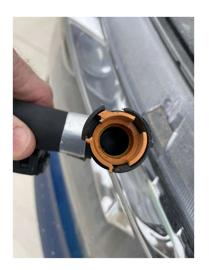
This removal will break the (3) locking tangs on the Orange connector. This is normal and necessary to remove the tamper-proof connector from the camcover spigot.
