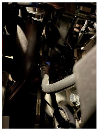
Lightly lubricate inner O-rings with engine oil and firmly connect lower PCV tube connector to induction tube spigot.
