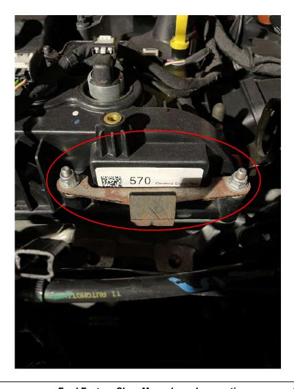
Remove vacuum line retainers from camcover studbolts, then install bracket over camcover studbolts and install (2) nuts.
