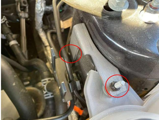
**Position bracket as shown and install pushpin through bracket into existing hole in strut tower (just below brake lines). Install M6 locking nut onto coolant reservoir studbolt and torque to 8Nm or 71 in\*lb.**
