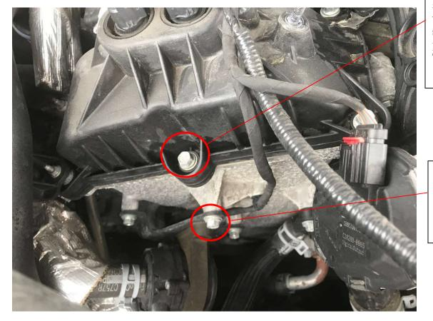
On passenger side of engine, remove camcover bolt and replace with camcover studbolt provided. Torque to 10nm (88 lbin)
