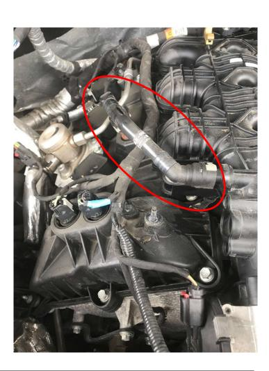
Remove existing PCV tube by releasing the tab on the connectors and pulling upward.
