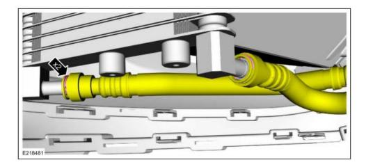
NOTE: After oil cooler installation, oil fill capacity will increase 0.5 qts.
