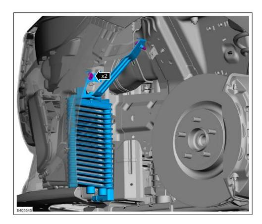
7. Connect the oil cooler tubes and install the retaining clips.
