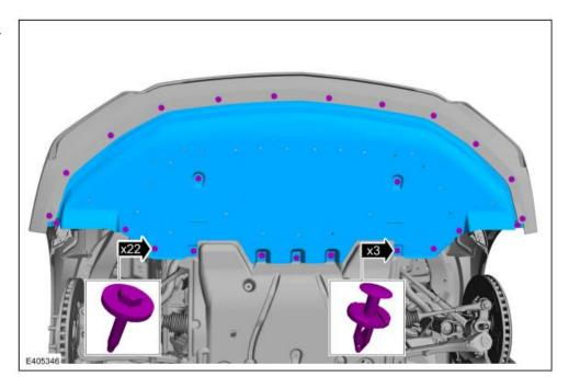
Remove the retainers, the bolts and the engine front undershield. Torque: 18 lb.in (2 Nm)
