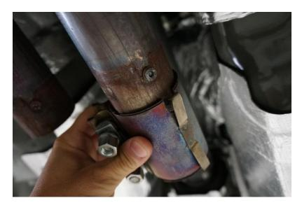
Step 7: Allowing exhaust to hang down, remove rear mufflers from hangers by moving the exhaust system towards front of vehicle. Note: Have someone help with this step.
