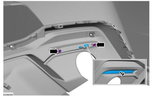
16. Remove the screws. Torque: 18 lb.in (2 Nm)
