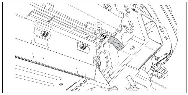
17. Install the left hand inner and outer bracket to the frame rail. Hand tighten the nuts at this time.
