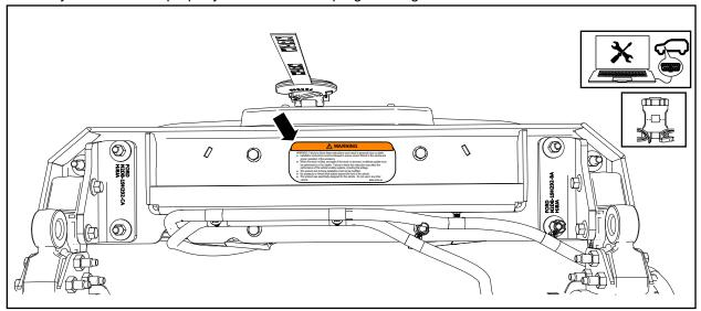
1. Remove the retainers and the skid plate.
