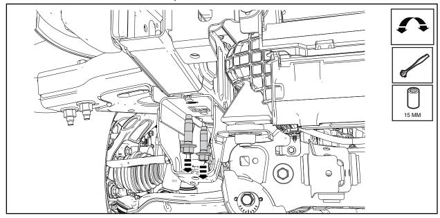
15. Install the winch CAC bracket and the bolts saved from step 14 to the frame.
