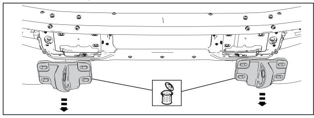
11. Remove the plastic holding nuts on both sides of the vehicle.
