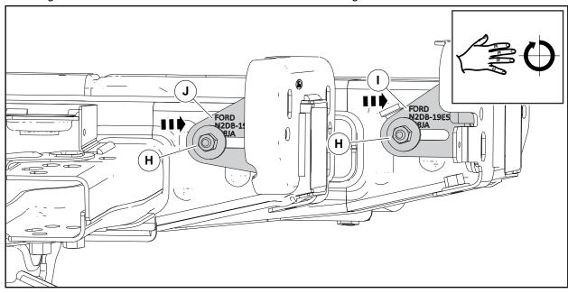
19. Install the frame rail bracket.
