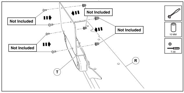
31. Install the winch mounting nuts into the winch housing slots.
