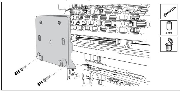
9. Remove the recovery hook holding bolts.
