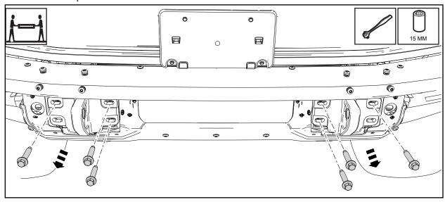
**NOTE:** If the bumper is equipped with a safari bar it must be removed before proceeding. The mounting bolts should be reinstalled and torqued to 18 lb.ft (25 Nm).
