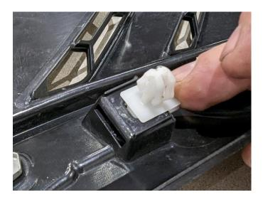
Step 5: Install (4) hood vent T-Studs into the carbon fiber hood vent in the locations noted in Step 3 by clipping them into position.
