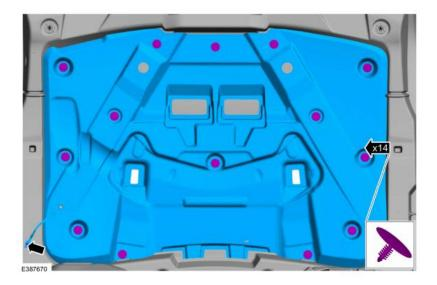
Step 3: Remove the nuts, the trim pins and the hood scoop. Remove any remaining 2 sided tape from the hood surface by rolling off with thumbs.
