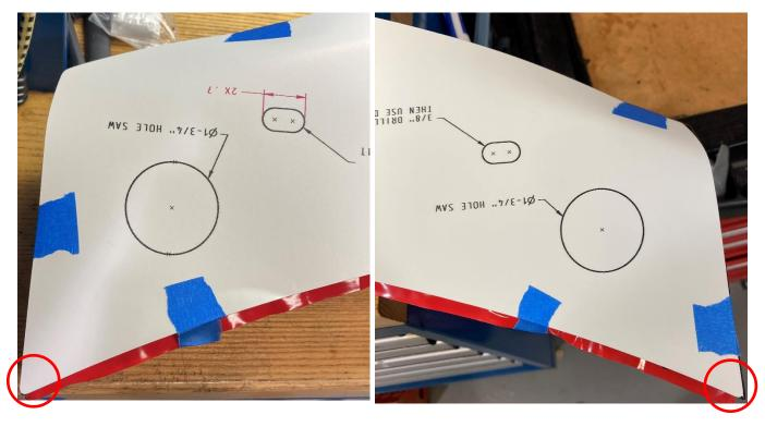
2. Securly tape down the edges of the template to the lower spoiler assembly.
