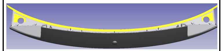
11. Remove the protective backing from the tape on the spoiler and install the spoiler to the lower spoiler assembly.
