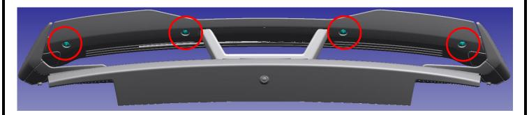
13. **NOTE:** When installing the spoiler, apply approximately 15 lbs. of pressure along the length of the spoiler to ensure adhesion of the two-side tape.
