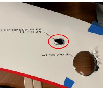
7. Use a 1 3/4" hole saw to drill the larger holes on the left and right side.
