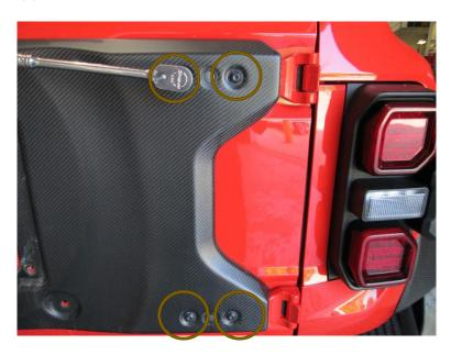
Step 6: Install the supplied accessory plugs into the carbon fiber exoskeleton.
