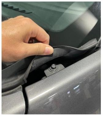
2. Position the vehicle mount bracket in place and reinstall the bolt, do not tighten yet.
