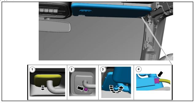
4. Open the fastener cover, remove the fastener and the sun visor clip. Perform this step on both sides.
