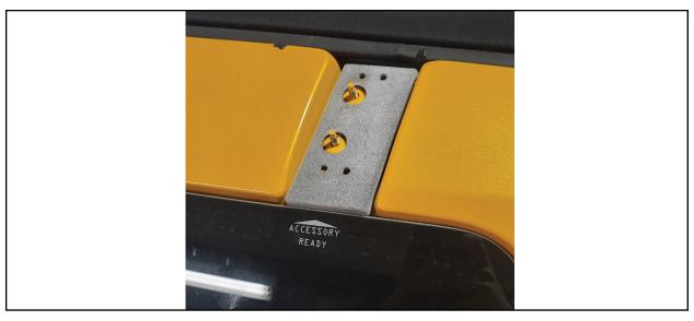
NOTE: The roof line brackets should be installed with the light bar mounting slot facing outward
