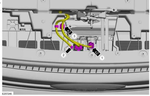
3. On both sides, remove the 2 screws. Torque: 15 lb.in (1.7 Nm)
