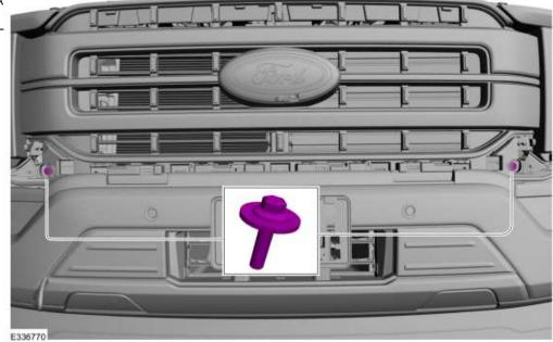
7. Remove the pin-type retainer. Pull up to disengage the locating pins along the top of the grille. Pull forward on center of the grille to remove.
