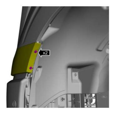
4. Remove the front bumper upper cover trim panel using a flat-blade screwdriver to release the locking tabs.
