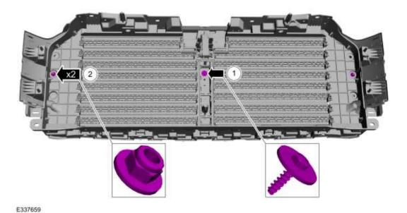
5. Separate the active grille shutter from the radiator grille.
