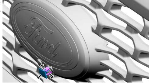
2. Remove the screws and the front camera washer and bracket as an assembly.
