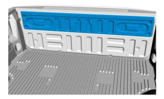
Use pliers to undo clips on the rear of the oval and remove from the tailgate.
