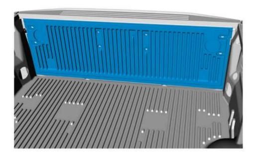
3. Remove the screws from the inner panel. *Torque*: 28 lb.in (3.2 Nm)
