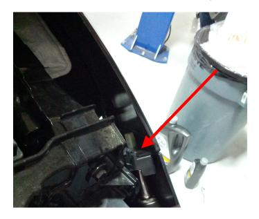
STEP 10: Remove front bumper cover by pulling corners gently out of fenders and by lifting plastic tabs. Carefully set aside on a soft surface to avoid scuffing the paint.
