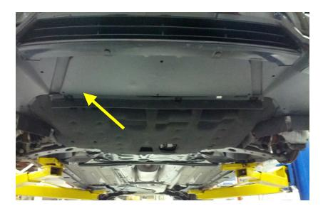
STEP 5: Remove 13 push pins from the lower front bumper splash pan, remove splash pan and set aside.
