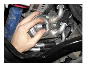
**STEP 14:** Tighten and torque the new threaded fitting to 58 Nm (43 lb-ft).
