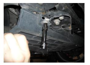
**STEP 18:** Reinstall under tray to front bumper cover with (9) bolts.
