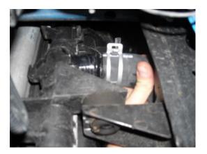
**STEP 12:** Install the oil cooler line bundle onto the oil cooler by firmly clipping the quick connect couplings onto the oil cooler.
