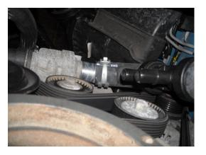
**STEP 11:** Install the new lower radiator hose onto the radiator and release the hose clamp.
