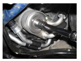
**STEP 15:** Install the oil cooler line bundle onto the lower radiator hose by firmly clipping the quick connect couplings into place.
