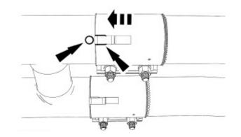
**STEP 5: NOTE:** Make sure to correctly align the exhaust H-pipe to the catalytic converters and intermediate pipes before tightening the fasteners.
