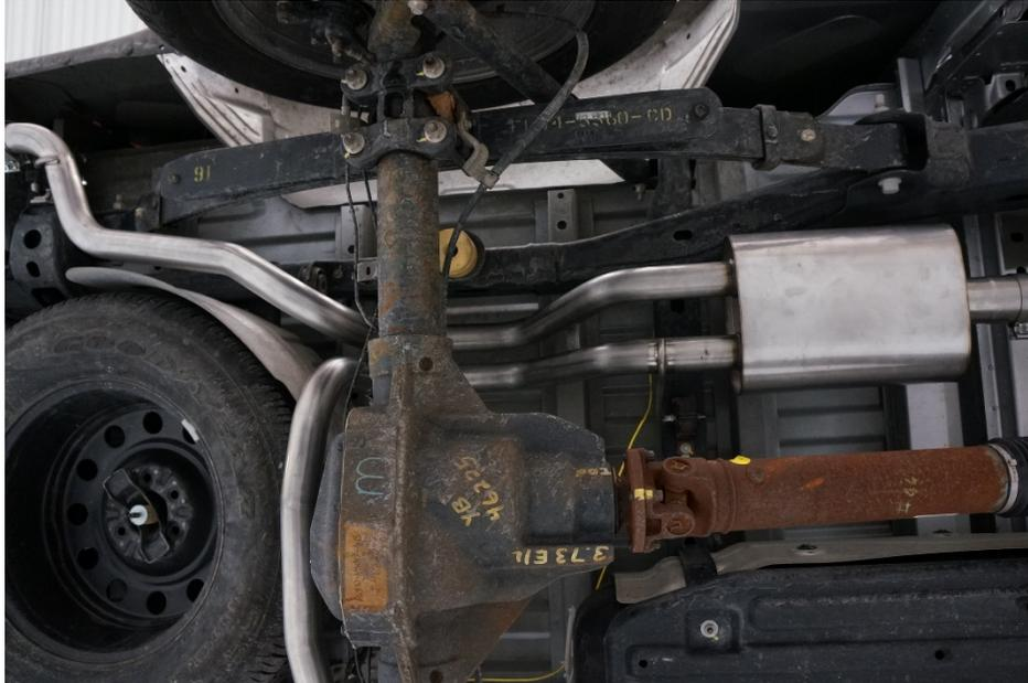
**Note: For vehicles with a 141" wheel base, cut 4" off front pipe.**
