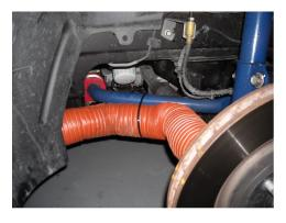
**STEP 13:** Slide the brake hose over the new backing plates and secure with provided hose clamp.
