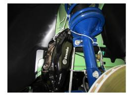
**STEP 10:** Remove the front rotors. Remove (3) bolts on the backing plate and remove.
