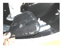
**STEP 5:** Insert the new bezel duct and attach using the (3) screws per side of vehicle.
