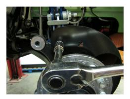
STEP 12: Install the provided tie wrap to fasten the brake duct hose to the anti-roll bar. Removal of the
