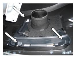
STEP 6: Using side cutters, snip the retaining wire on brake duct hoses at both ends two to three wires inboard. Then gently pull the wire from the end of the hose to remove.
