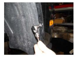
**STEP 5:** Remove (2) upper fascia bolts and (4) grill retaining clips.
