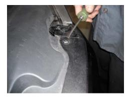
**STEP 6:** Unclip the ambient air temperature sensor in the lower grille from fascia.
