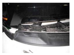
**STEP 18:** Place templates on top side of lower grill insert and transfer hole locations.
