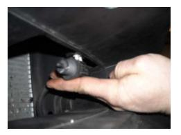
**STEP 26:** The lower grill insert has (8) locations on leading edge for additional clips as highlighted below.
