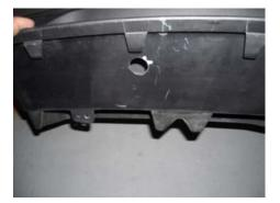
**STEP 20:** Remove the (4) bottom clips on the leading forward edge of the splash guard.
