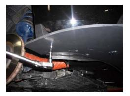
**STEP 35:** Install the upper splitter rod end through the lower grill insert and thread into bumper bracket.
