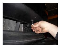
**STEP 36:** Install the splitter support rods onto rod ends; torque bolts through splitter to 28 in.-lb.
