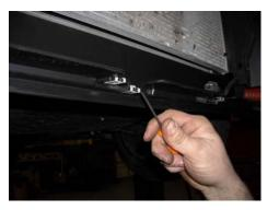
**STEP 21:** Replace the removed clips with the (4) J-Nuts provided in Splitter Kit M-16601P-MB.
