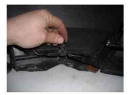
**STEP 17:** Gently unclip lower grill insert from fascia and remove by sliding forward.
