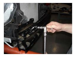
**STEP 14:** Install (4) nuts on rear side of bumper bolts and tighten down onto the splitter bracket to 18 ft.-lb.
