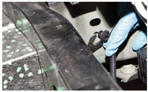
STEP 26: Feed the horn loom back under the headlight - towards the wheel arch liner
