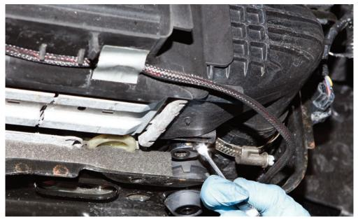
STEP 15: Disconnect the horn plug as shown
