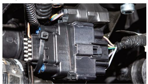
STEP 25: Using a trim tool, or similar, free the locating mount for the horn loom
