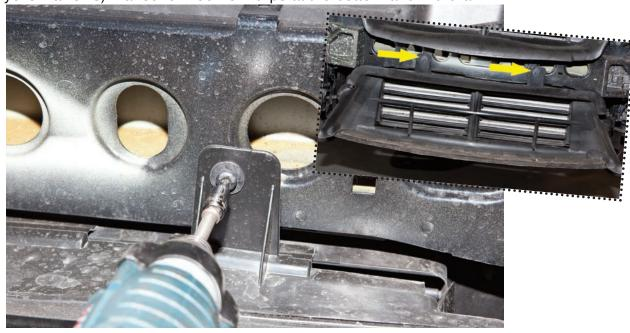
STEP 11: You'll now have access to the 'active grill shutter' - this needs to be removed later but at this point push the blades to ensure it's in the fully closed position
