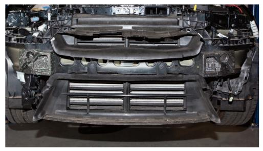
**STEP 9:** Pull the top air duct free from its mounting locators
