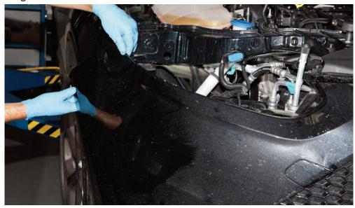
STEP 8: You'll need two people to withdraw the bumper assembly - you'll need to disconnect the fog light (located on RHS) before the bumper can be fully removed
