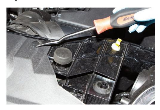
STEP 2: Disconnect the bonnet release cable and then withdraw the top cover
