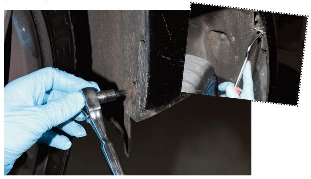
STEP 6: A) Undo and remove the lower deflector B) Remove the rear section of the undertray C) Undo and remove the corner deflector as shown
