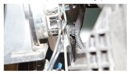
STEP 17: Undo the horn bracket mounting bolt and withdraw the horn assembly
