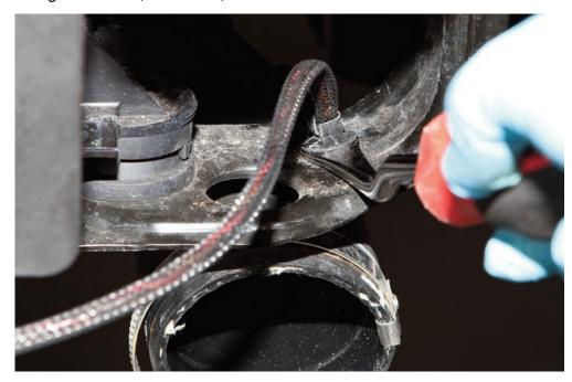
STEP 23: Manouver the AGS free of the two clips on either side and then remove the complete assembly
