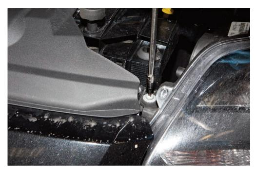
Pull the headlight's upwards to remove it from its mount. You'll need to disconnect the plug as shown
