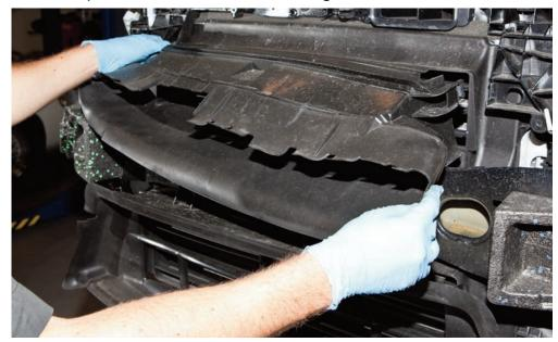
STEP 10: Undo the two torx screws holding the lower air duct (as indicated by the yellow arrows) manouver free from clips at the bottom and withdraw
