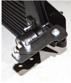
**STEP 21:** Disconnect the active grill shutter connector shown
