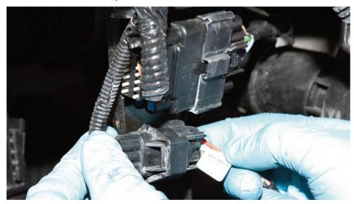
STEP 22: Using a trim tool, or similar, free the AGS loom
