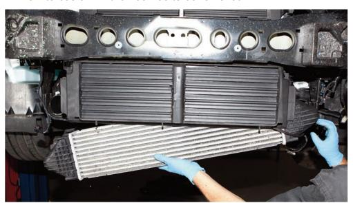
STEP 19: Remove the MAP sensor from the end of the intercooler
