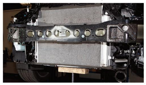
STEP 28: Remove the radiator cradle bolts on both sides
