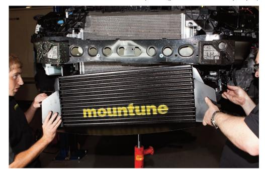
STEP 30: The side brackets fit underneath the radiator cradle as shown in STEP 30 and 31
