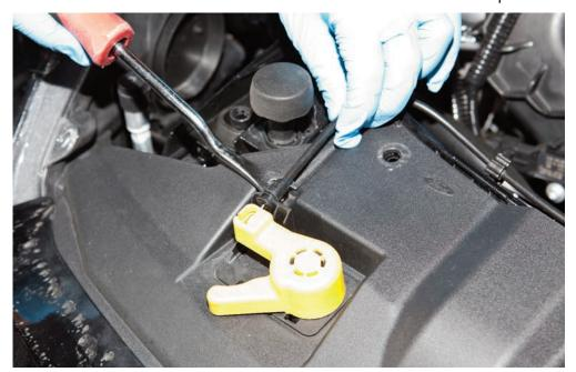
STEP 3: Remove the two headlight locating screws on both headlights
