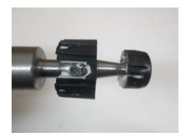
**STEP 28:** Verify the hole for the reverse lockout shoulder bolt is orientated towards the driver side of the shifter housing.
