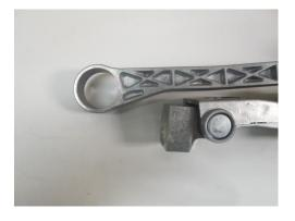
**STEP 41:** Install the new front isolator bushings by sliding them into the front arm.
