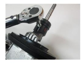
**STEP 35:** Install the spring over the shifter lever.
