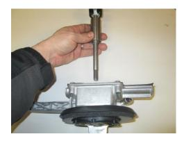
STEP 25: Apply a liberal amount of supplied grease to the new shifter lever pivot and pivot isolator bushing.
