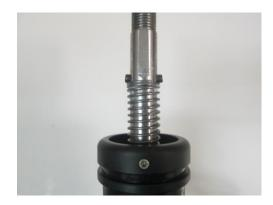
STEP 37: Install the inner dust boot. Ensure the upper portion of the boot slides into the machined groove on the reverse lockout. Also verify the lower portion of the boot fits securely around the shifter assembly base.
