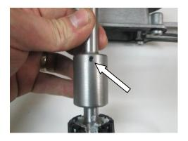
STEP 29: Slide the new shift lever into the housing, once again, verify the reverse lockout shoulder bolt hole is orientated towards the driver side of the shifter housing.
