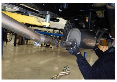
**STEP 2:** Insert the front and rear hangers into the isolators.
