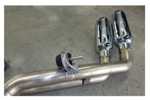
**Step 4:** Slide (2) 2.25" clamps over the expanded tailpipe inlets then slide both expanded inlets over the muffler outlet pipes. Snug the clamps do not tighten!
