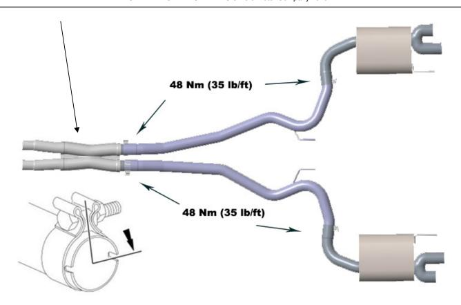
Tighten the exhaust clamp.
