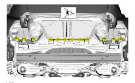
Step 24: If required, remove the screws and the side bracket.
