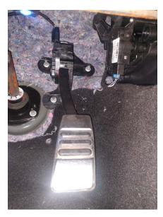
STEP 3: Connect the accelerator pedal electrical connector. Secure by depressing the RED locking retainer.
