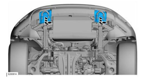
Remove the bolts and the front tow hook assemblies.
