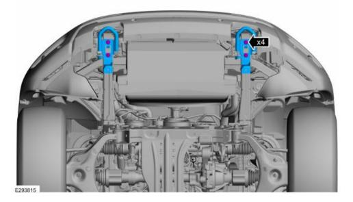
Install new tow hooks. Apply thread locking compound to bolts *Torque*: 46 lb.ft (62 Nm)
