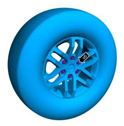
MARNING: Retighten wheel nuts within 160 km (100 mi) after a wheel is reinstalled. Wheels can loosen after initial tightening. Failure to follow this instruction may result in serious injury to vehicle occupant(s).
