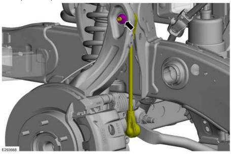
Position the tie rod end and install the new tie rod end nut.
