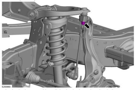
Position the brake hose and install the brake hose bracket bolt.
