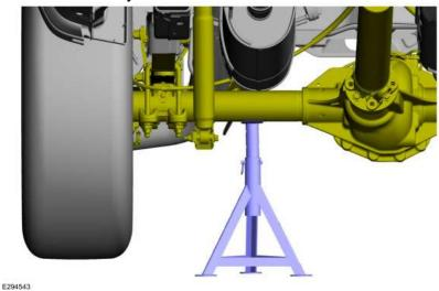
Remove and discard the rear shock absorber upper and lower bolts and nuts. *Torque*: 52 lb.ft (70 Nm)
