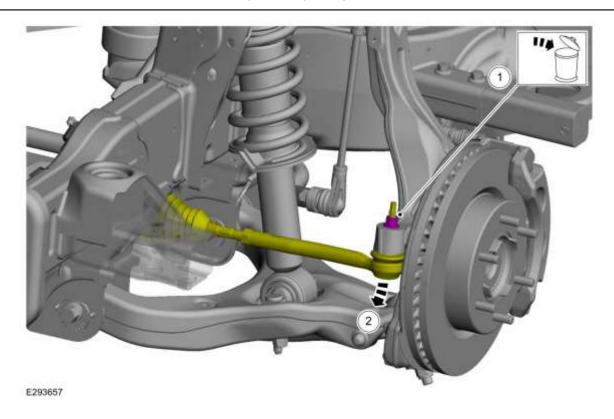
Loosen the upper arm ball joint nut, do not remove nut completely.
