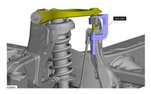
Remove and discard the shock absorber and spring assembly lower nuts.
