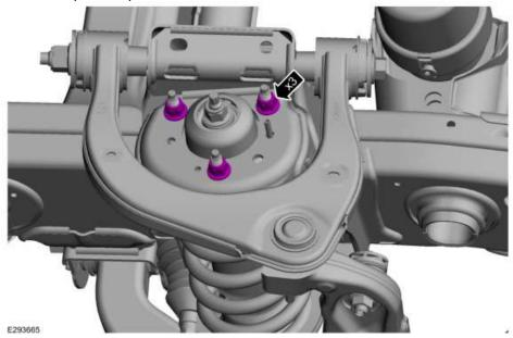
Install the new shock absorber and spring assembly using 2 supplied bolts and washers. Apply blue medium strength thread locking compound, install bolts from below through control arm into shock assembly.
