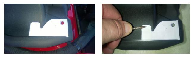
Step 5. Cut 1" hole with center in the marked location. A 1" drill or 1" hole saw may be used.
