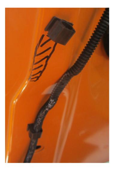
Step 10. Release both clips. Remove hose from both clips. Move hose downward about 1/2" Re-fasten lower clip. Interference area as marked. (2018 only)
