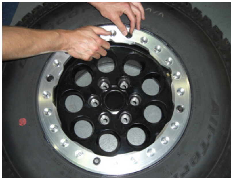
Pic 5.2 – Tighten each bolt at least 1 full turn with a socket wrench
