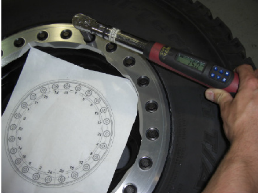
Pic 7.2 – Torque in the proper sequence using a torque wrench.
