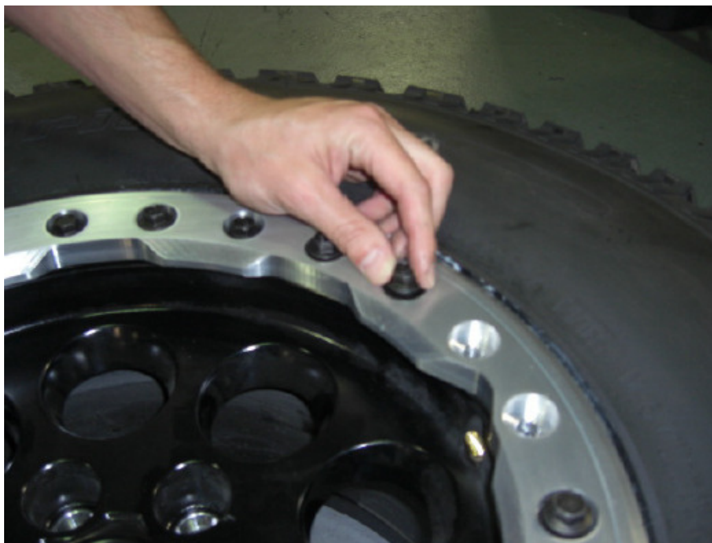
Pic 6.1 – Hand thread in all remaining bolts.
