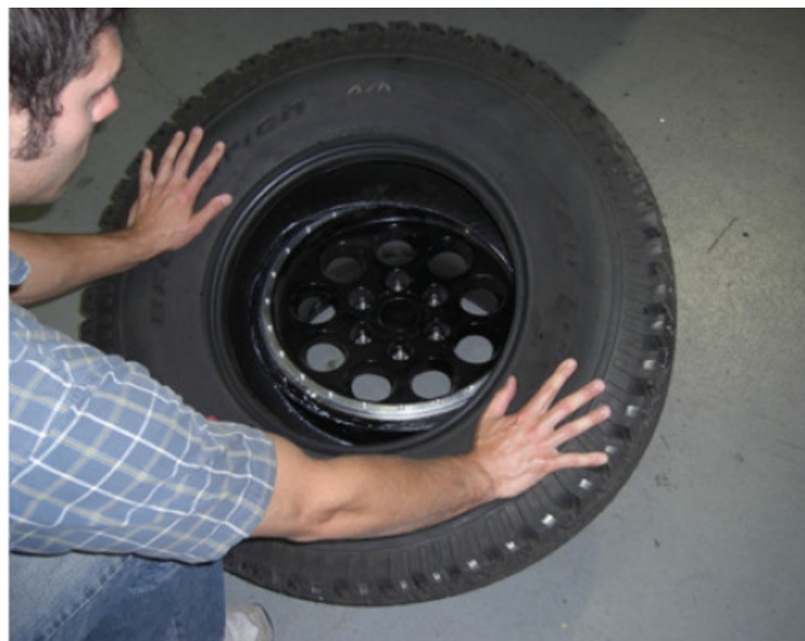
Pic 2.1 – Force the inner tire bead over wheel flange
