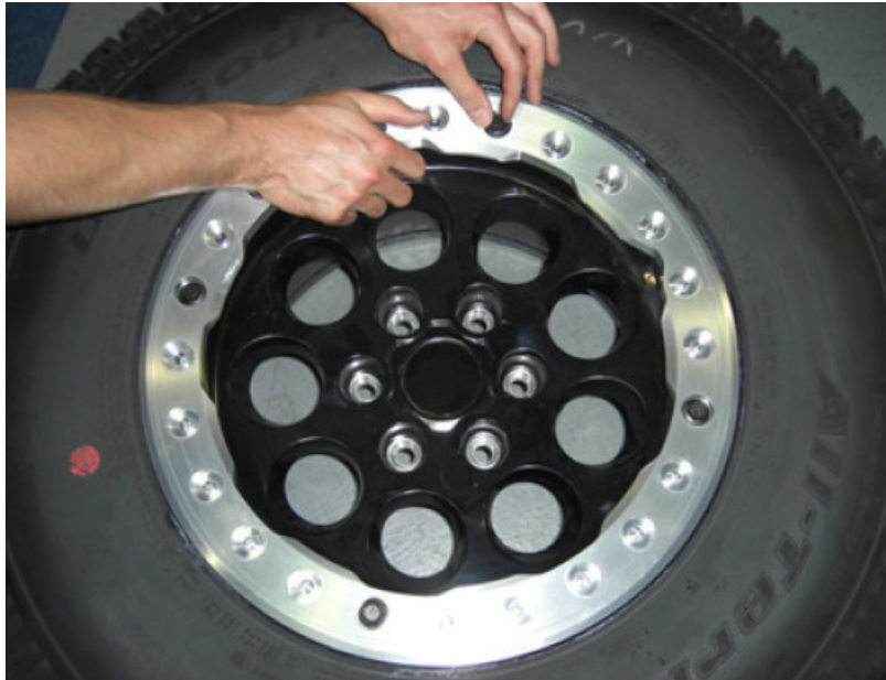
Pic 5.1 – Hand thread 4 bolts at the corners.
