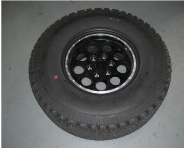
Pic 3.1 – Outer tire bead fits on wheel flange
