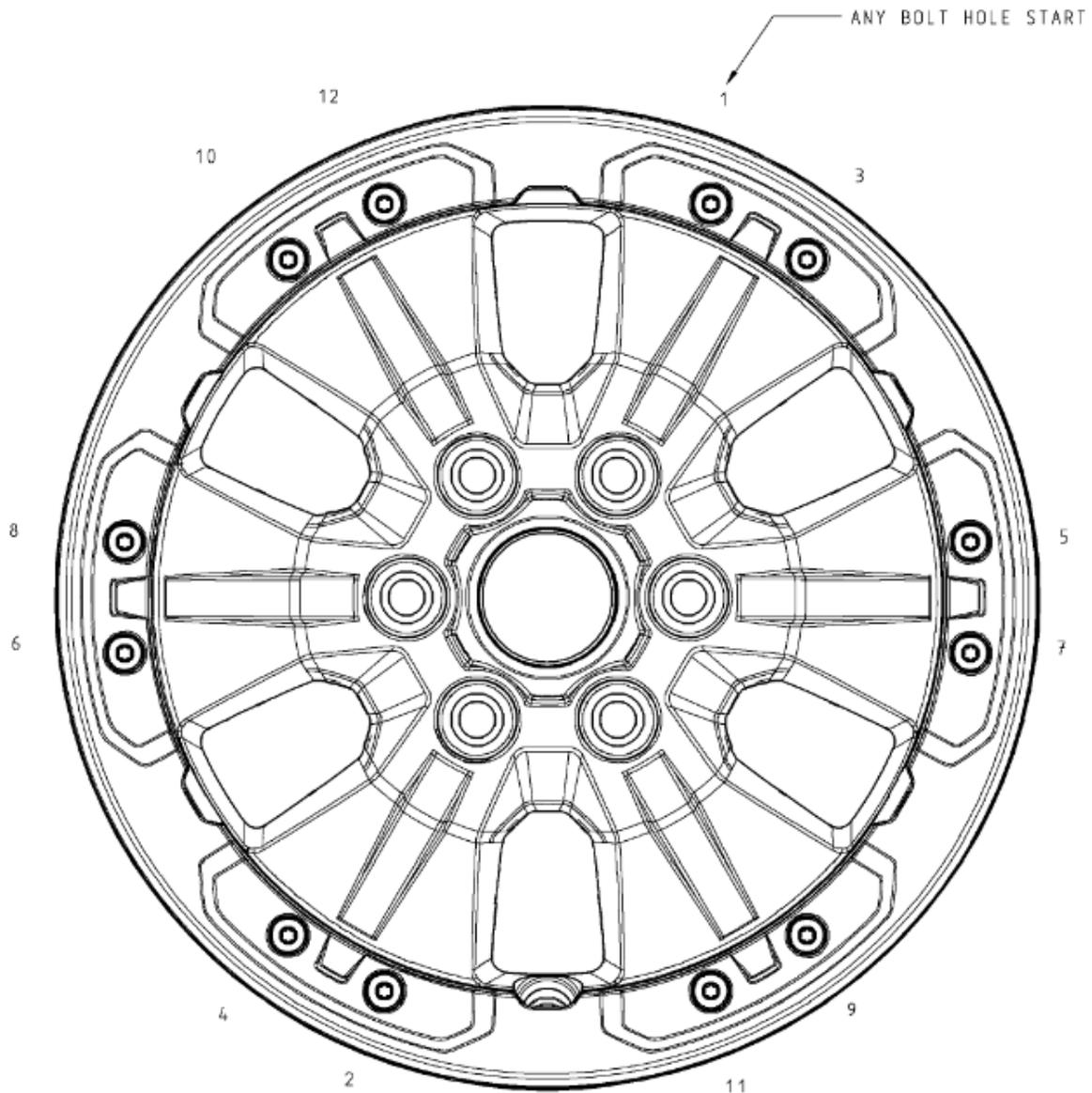
**Step 1.** Hand tighten all bolts in sequence. **Step 2.** Final torque in sequence 17.5 N.m.
