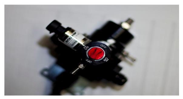
Taking a sample will require a length of 5/32" fuel proof rubber hose to reach whatever vessel being used to hold the sample. After installing the sample hose, with the vehicle master cutoff switch on, turn on the
