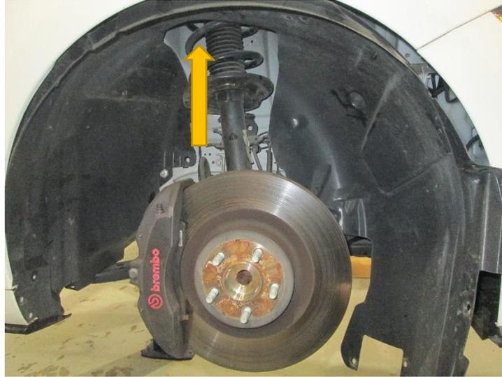
**STEP 22:** Position the wheel and install the wheel nuts. Tighten the wheel nuts in a star pattern. Torque to: 148 lb.ft (200 Nm)
