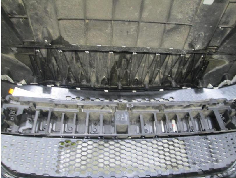
**STEP 16:** Slide the fascia assembly onto the front of the vehicle. Install the (2) outer fascia mounting screws. Torque to 18 lb.in (2 Nm). Install the (6) remaining fascia mounting screws. Torque to 53 lb.in (6 Nm)
