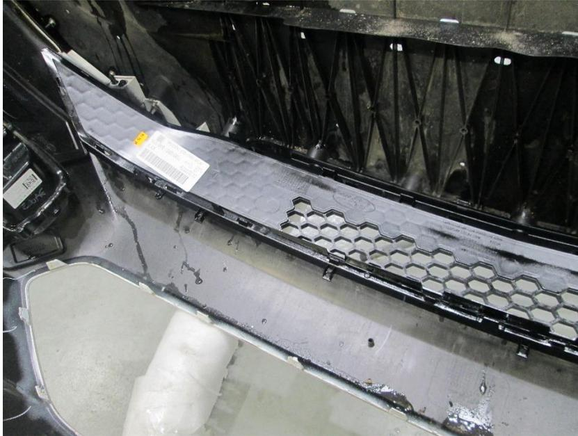
**STEP 14:** Place the new upper grille on the fascia. Starting from the center and working outboard, align the fascia clips with grill mounting provisions and gently clip the grille into the fascia.
