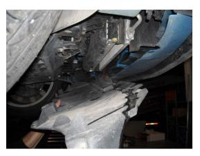
**STEP 3:** Loosen valve on radiator and drain the engine cooling system.
