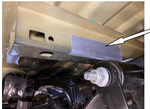
PROTECTIVE TAPE APPLIED ON THE REAR OF THE CROSSMEMBER ABOVE THE SPRING SHACKLE
