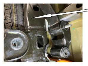
UPPER SHACKLE BOLT BEING REMOVED OVER THE TOP OF THE FRAME
