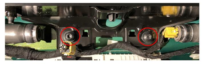
Install the C-bow brace to the side pillars using the bolts and washers (M8x30).
