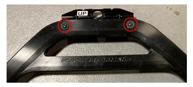
2. Install the J-clips (M8) on the rear header, as shown in the image.
