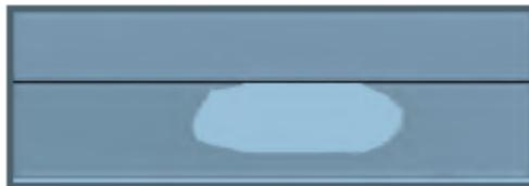
4. For halogen or LED headlamps: On the wall or screen you will observe a light pattern with a distinct horizontal edge toward the right. If this edge is not at the horizontal reference line, you will need to adjust the beam so the edge is at the same height as the horizontal reference line.
