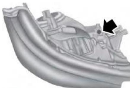
5. Locate the vertical adjuster on each headlamp. Use a #2 Phillips screwdriver to turn the adjuster either counterclockwise or clockwise in order to adjust the vertical aim of the headlamp.
