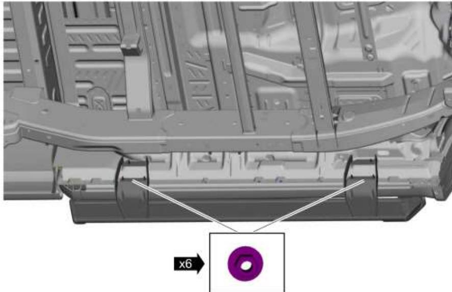
3. Remove the running board assembly.
