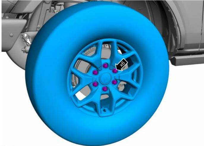
**Step 28:** Install the wheel nuts. For Bronco Raptor (M14 Wheel Stud), tighten to 200 Nm (147.5 lb-ft).
