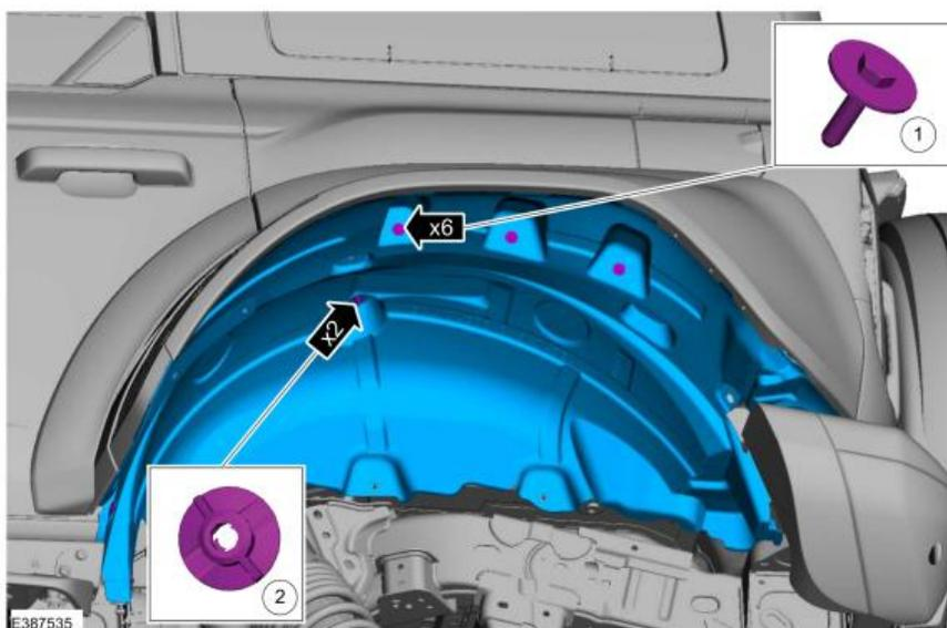
**Step 6:** Loosen the wheel molding bracket.
