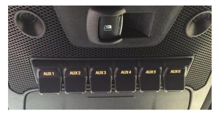
Note: This kit will use 3 of the in-vehicle upfitter switches. Disconnect the (-) Negative Battery Terminal connection to the vehicle.
