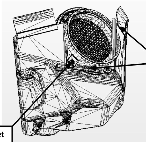
**STEP 4:** Lower the complete air intake bucket assembly into the vehicle using the two pegs as guides into the rubber grommets. Use the new air intake bucket bolt and newly supplied J-clips to secure the air intake bucket in the vehicle. Torque the M6 bolt to 8 Nm (70 lb in).
