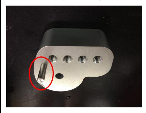
**STEP 8:** Install adaptor onto front cover as shown. Torque fastener to 30 Nm.
