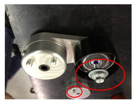
**STEP 18:** Install single-pin tensioner adaptor onto tensioner sub-assembly. Install fastener through center hole. Torque fastener 40 Nm.
