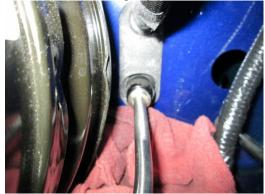
**STEP 12:** From the underside of the vehicle, push the hydraulic hose retaining clip back into the elbow.
