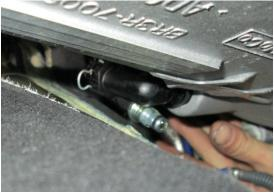
**STEP 9:** From the topside of the vehicle, carefully feed the hydraulic clutch line out of the vehicle.
