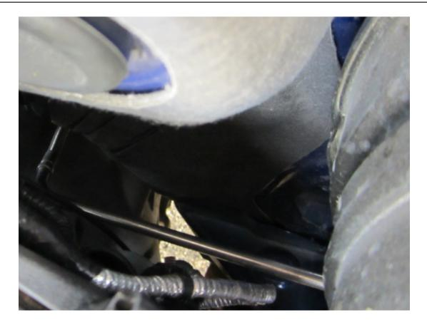
**STEP 11:** Push the hydraulic hose retaining clip back into the housing.
