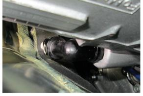
**STEP 13:** Feed the new hydraulic clutch line down the elbow on the transmission housing, lubricate the O-ring and gently push the new hydraulic clutch line end into the clutch cylinder housing until it locks into the retaining clip
