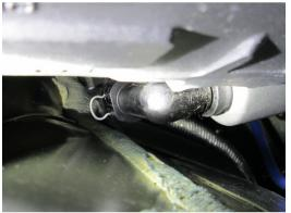
STEP 8: Gently pull the hydraulic hose out of the transmission elbow.
