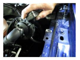
**STEP 3:** Remove the intake tube from the fire wall by gently pulling towards the front of vehicle, then place to the side.
