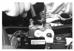
STEP 10: Remove the shifter from the car.
