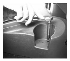
**STEP 2:** Remove the rear cup holders. Squeeze the center and pull forward to undo the back tab, then pull straight up to unsnap the cup holder. Remove the nuts holding the rear of the console.
