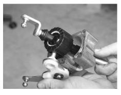
**STEP 12:** Remove the black rubber sheath from around the plastic pivot cup on the shift lever. Then separate the two halves of the plastic pivot cup and remove them from the shifter.
