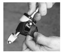
**STEP 15:** Transfer the plastic bushing from the short side-lever on the stock shifter to the new shifter.
