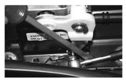
**STEP 9:** Remove the four screws from the top of the shifter with a **T-30 Torx** bit. **Hold the bit straight and apply downward pressure to prevent stripping the shallow Torx screws**. The screws are coated with thread-locking compound, so they will be hard to turn.
