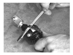
**STEP 13:** Grease the large pivot ball in the middle of the new shifter with the grease provided.
