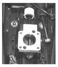
**STEP 18:** Lower the new shifter down onto the shifter base and install the new 6mm socket head bolts provided. Tighten bolts with a 5mm Allen wrench.
