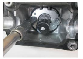
**STEP 31:** Apply a liberal amount of supplied grease to the lower actuator arm and bushings. Align actuator arm bushings into the shifter housing and lower shifter pivot.
