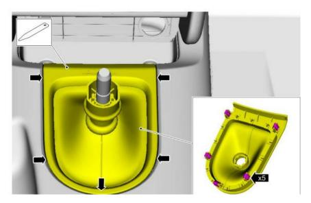
**STEP 4:** Release the retainers and remove the gearshift lever boot.
