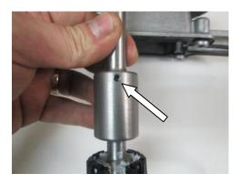
**STEP 29:** Slide the new shift lever into the housing, once again, verify the reverse lockout shoulder bolt hole is orientated towards the driver side of the shifter housing.
