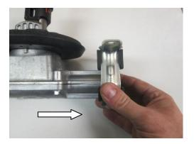
**STEP 16:** Remove anti rattle clip for the shifter lever if equipped.
