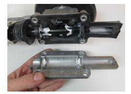
**STEP 22:** Remove the lower actuator arm by slowly lifting off of the lower shifter lever pivot.
