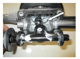
**STEP 23:** Remove (2) bolts from shift lever retaining plate. Remove plate.
