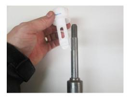
**STEP 20:** Separate the dust boot from lower shifter housing. Remove (4) lower housing retaining bolts.
