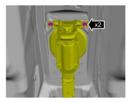
**STEP 45:** Raise the transmission back into place and install (4) bolts using Blue thread locking compound. Torque: 46 lb.ft (63 Nm)
