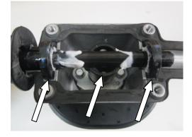
**STEP 32:** Install the provided housing gasket onto the shifter assembly. Slide the lower housing cover into place. Install (4) bolts with Blue thread locking compound. Torque: 75 lb.in (8.5 Nm)
