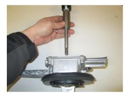
**STEP 25:** Apply a liberal amount of supplied grease to the new shifter lever pivot and pivot isolator bushing.
