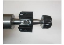
**STEP 28:** Verify the hole for the reverse lockout shoulder bolt is orientated towards the driver side of the shifter housing.
