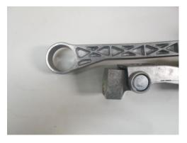
**STEP 41:** Install the new front isolator bushings by sliding them into the front arm.
