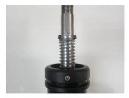
**STEP 37:** Install the inner dust boot. Ensure the upper portion of the boot slides into the machined groove on the reverse lockout. Also verify the lower portion of the boot fits securely around the shifter assembly base.
