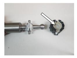
**STEP 26:** Slide the pivot isolator bushing over the shift lever pivot ball.
