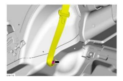
8. Install the retainers and the safety belt retractor. *Torque*: 30 lb.ft (40 Nm)
