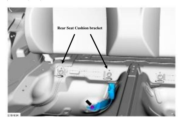
**NOTE:** During installation, make sure the safety belt webbing is not twisted and the safety belts and buckles are accessible to the occupants.
