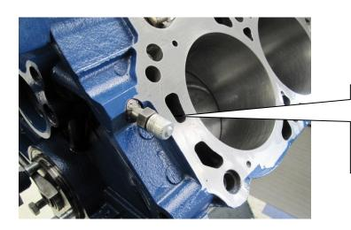
Oil pressure available at the right rear of block via -4 AN fitting with an O-ring seal.
