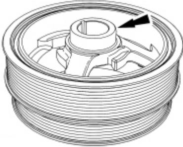
Using the Crankshaft Vibration Damper Installer, install the crankshaft pulley.
