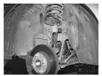
STEP 2: Remove caliper and support to avoid damage to the line. Remove rotor for additional clearance
