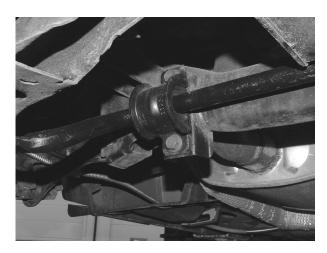
STEP 4: With floor jack located under lower control arm, compress right side spring.
