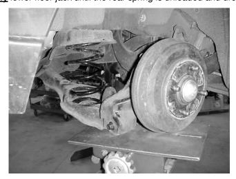
STEP 8: Place new rear spring (item 1) in place, raise floor jack until lower control arm to knuckle bolt can be
