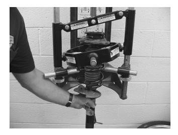
STEP 7: Assemble SVT strut-spring assembly using the following new items; front strut, RF (item #4), bump
