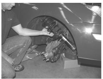
!!! Warning: Spring is under extreme compression. To avoid personal injury use a suitable spring compressor!!!
