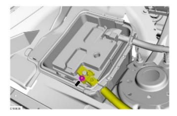
3. Position the positive battery cable cover, loosen the nut and position the positive battery cable. *Torque*: 44 lb.in (5 Nm)
