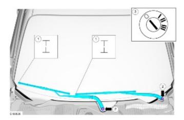
3. Install the windshield wiper pivot arm nut covers.
