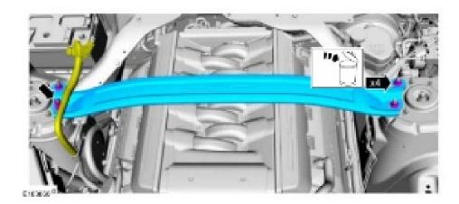
3. Remove the fasteners and the cowl extension.
