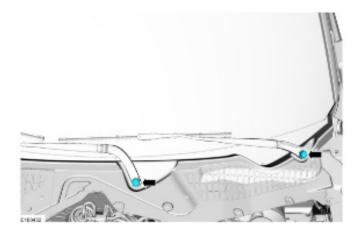
2. Remove the windshield wiper pivot arm nuts. *Torque*: 26 lb.ft (35 Nm)
