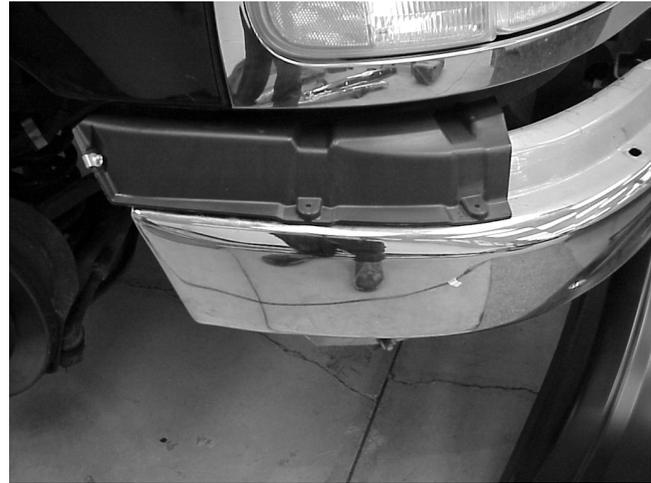
**STEP 8:** Install left and right lower bumper brackets with the fasteners supplied as shown in the figure below.
