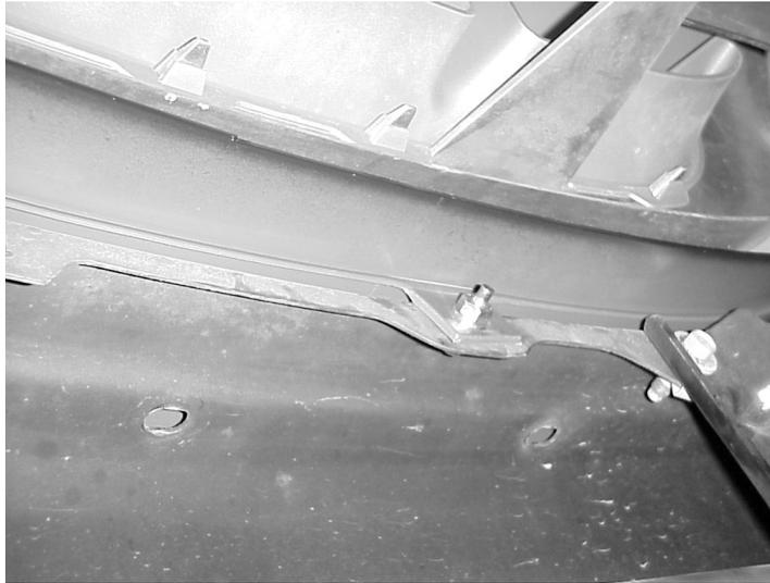
**STEP 12:** Attach fascia support to lower fascia with supplied fasteners as shown in the figure below.
