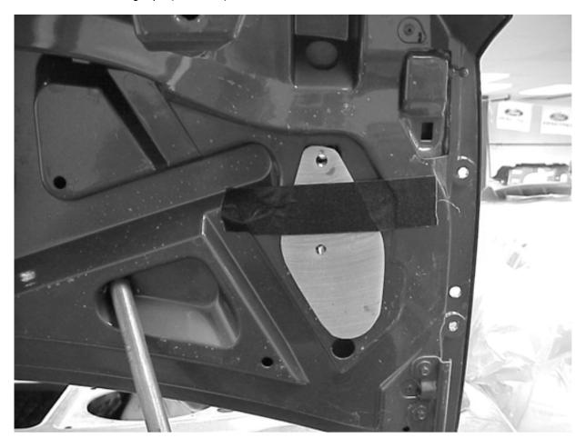
**STEP 3:** Mark the center of each hole with a center punch or marker.
