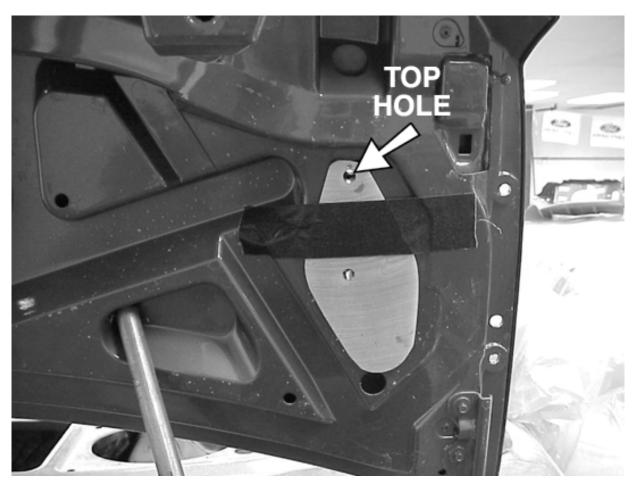
**STEP 6:** Fill the cavity between upper and lower deck lids through the *top* hole using the 5 minute epoxy.
