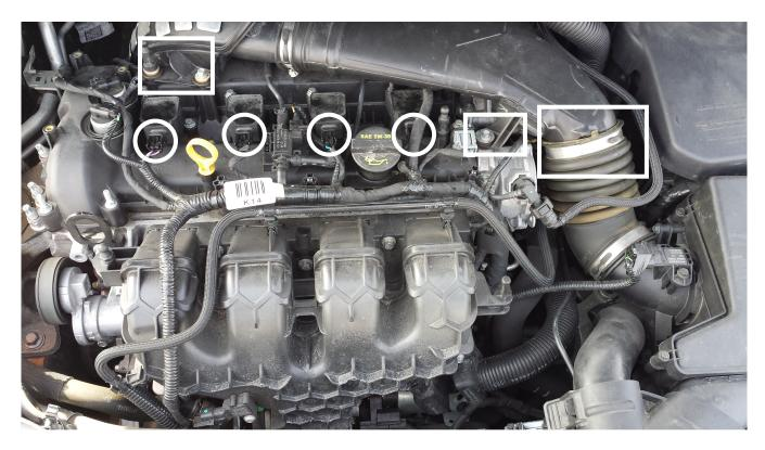
Address the components enclosed in rectangles above. Use the flathead screwdriver to loosen the clamps on the section of intake covering the plug coil. Remove the bolt attaching the intake to the engine. Remove the section of intake and set aside.
